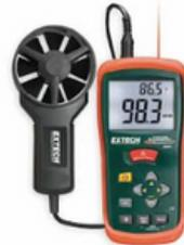
This instrument measures air velocity at a single point. To get an accurate reading of the velocity of air coming through a diffuser, you would need to imagine a grid over the diffuser, take measurements in each area of the grid and average them. Then multiply the average velocity (in feet per minute) x the area of the diffuser (square feet). You will measure the area of the diffuser in inches; then divide square inch area by 144 to convert it to square feet.
